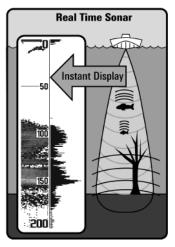
SONAR is an acronym for SOund and NAvigation Ranging. Sonar uses precision sound pulses or "pings" which are emitted into the water in a teardrop-shaped beam.
